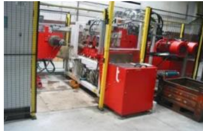
CNC Tube Forming & Bending (for key socket)
