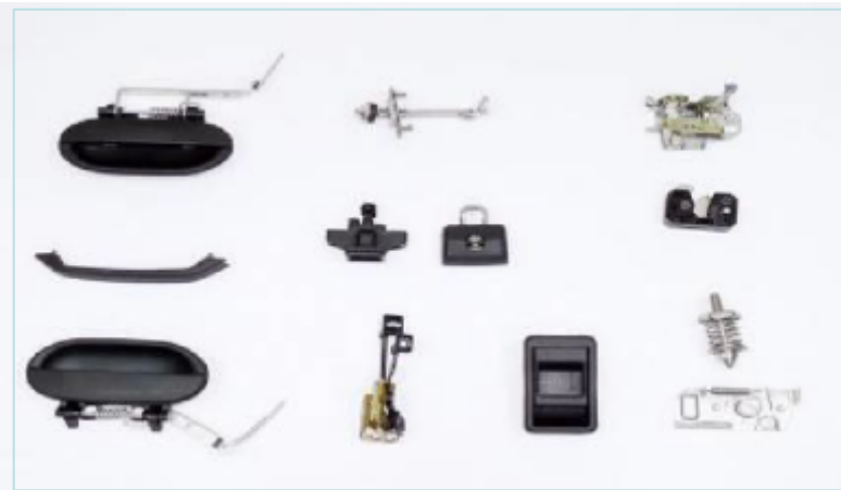
Door engine hood and rear hood latches and outside/inside mechanisms; Door stop
