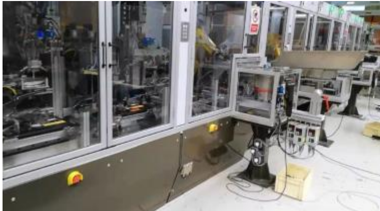
Automatic Assembly Lines Hand Brake
