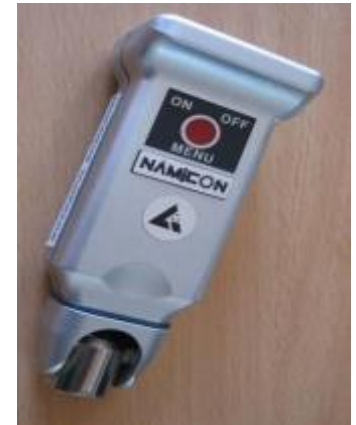
Zinc-coating thickness measurement NAMICON
